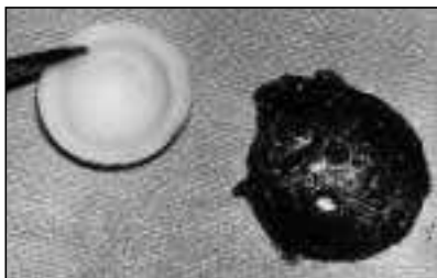
Fig. 3 Example of Type II cup. The retrieved specimen has extensive polyethylene wear and a broken polyethylene insert.
