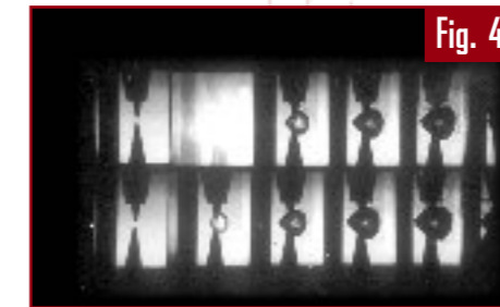
High-speed recording of a spark discharge (Frame rate: 2 x 10 6 frames per second). The spark ignition takes place in frame 2 of the upper row. A plasma bubble subsequently forms. A shock wave cannot be detected yet. It has already detached itself between the second frame of the first row and the second frame of the second row.
