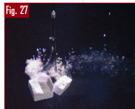
Effect of a focused shock wave on a cube-shaped artificial stone with an edge length of 10 mm. (Shock wave occurrence from the right). One can see the stone held on a wire, the fragmentation into a few pieces and cavitation bubbles in the shock wave path.
