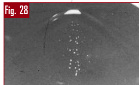
Cavitation bubbles created by a shock wave running from bottom to top. Directly behind the shock wave, the bubbles are still small. They grow within approx. 30 microseconds and then collapse while emitting a secondary (spherical) shock wave (circular rings at the bottom of the frame).
