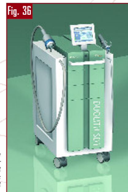
Combination device DUOLITH SD1 for generating and applying focused shock waves and unfocused pressure waves.
