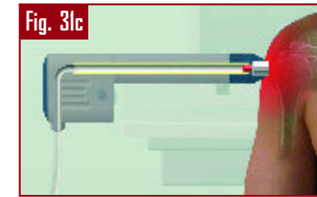
Phases of pressure waves generated by the impact of solid bodies on an impact body. The impact body transmits a pressure pulse into the coupled tissue.
