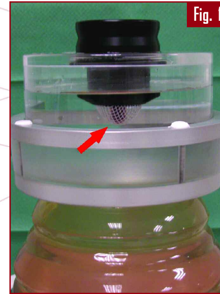
Standardized test set-up for the reproducible investigation of shockwave effects on bacteria in suspension. The arrow indicates the test probe located within the shockwave focus.
